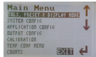
Raw counts are the digital outputs, ranging from approx., 20 to 4,095, that represent the position of the LVDT over its measurement range.
