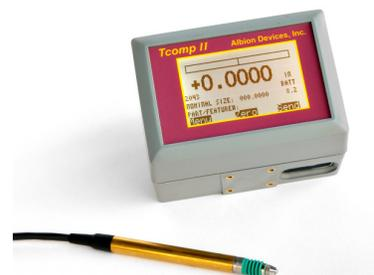
Available with LVDT only, for applications not requiring temperature compensation
